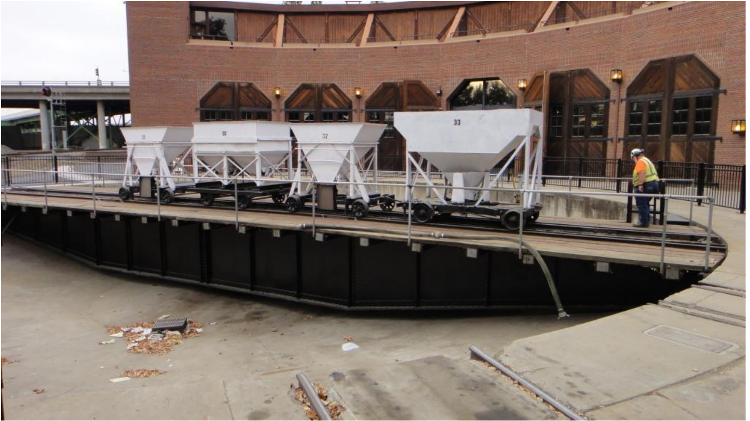
Frank spinning the ballast-hoppers 180 degrees on the turntable
