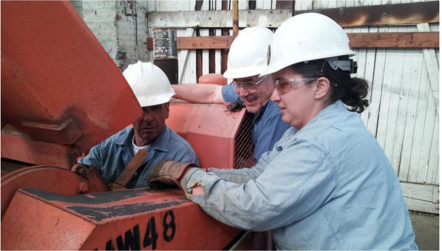
Mike T., Joe, and Heather install the new blades on the chipper
